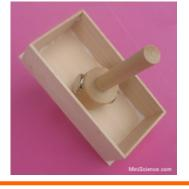
Make sure the box glue is dried and then insert the rotor in the hole of the bottom board. Now the magnet is completely in the box.
